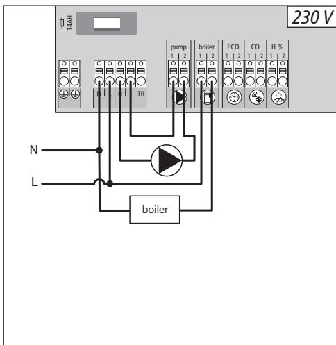
The boiler connection allows the control of a heat generator. Additionally, a pump can be controlled directly.
