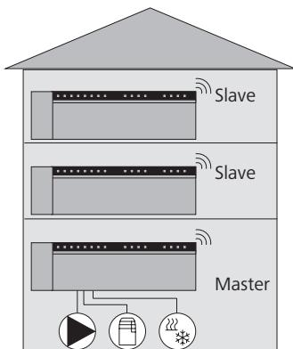
**Note:** The base station the components are connected to must be configured as master. Further base stations can only be paired with the master.
