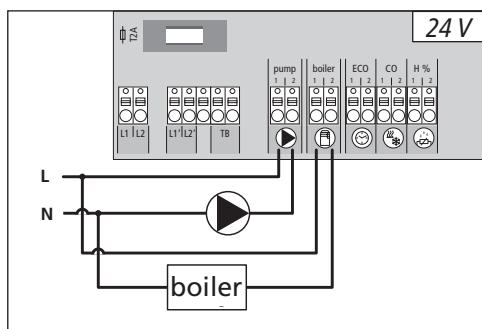
The boiler connection allows the control of a heat generator. Additionally, a pump can be supplied and controlled directly.
