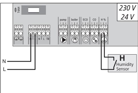
Humidity sensors (to be provided by the customer) serve for dewing protection in the cooling mode.
