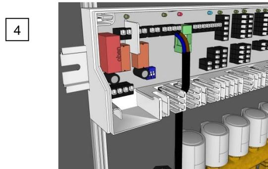
4 Lay the cable into the casing through the strain relief and install all cables to the basis using the clamping/plug-in technology; this is possible in a very short time.
