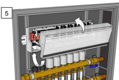
5 Close the cover and apply mains voltage. Now the basis is ready to operate.
