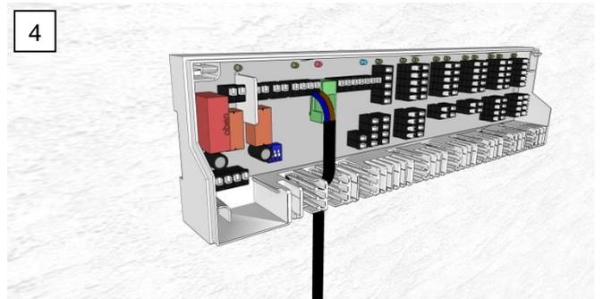
Lay the cables into the casing through the strain relief and install all cables to the basis using the clamping/plug-in technology; this is possible in a very short time.
