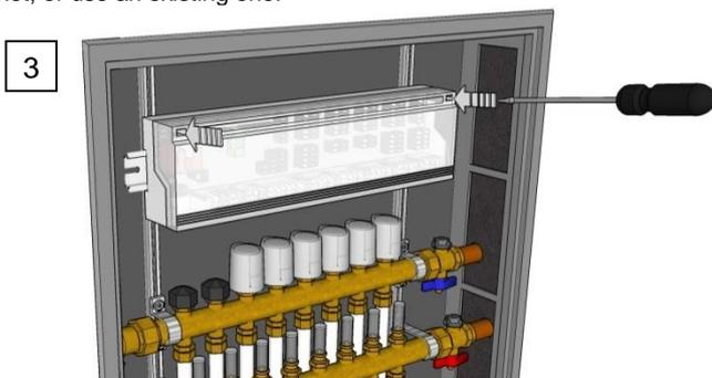
3 Loosen the casing cover at both latching points with a screwdriver and remove it.
