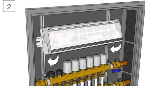
2 Position the basis slightly tilted onto the DIN rail and latch it in.
